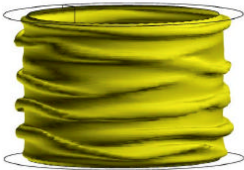
Figure 3: Three-dimensional time-dependant wavy spiral flow, Re_o = -500 , Re_i = 370 , h = 0.75 , L = 6 . Three-dimensional display of instantaneous isosurface of the azimuthal component of velocity, v = -1.6 \cdot 10^{-1} .
