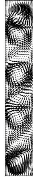
Figure 2: Three-dimensional time-dependent Wavy Vortex Flow, Re_o = -250 , Re_i = 750 , L = 6 , h = 0.75 . Instantaneous vector plot of velocity projected on an azimuthal plane ( r, z ).
